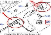
Front anti roll bar thickness bare metal is 19mm +/- 1mm, Anti roll bar links are 284mm in length +/- 1mm or 240 +/- 1mm. Front camber must not exceed 4°
